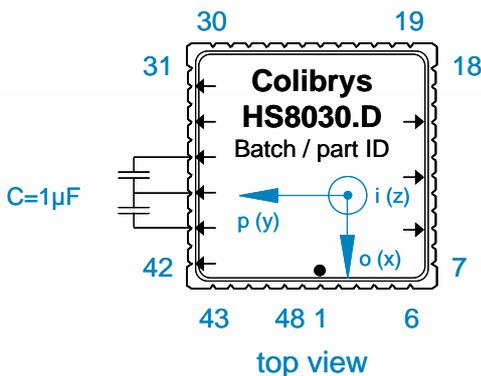
Each accelerometer is clearly marked with the manufacturers part number (i.e. HS8030.D), the batch number or lot number and the part ID number.
