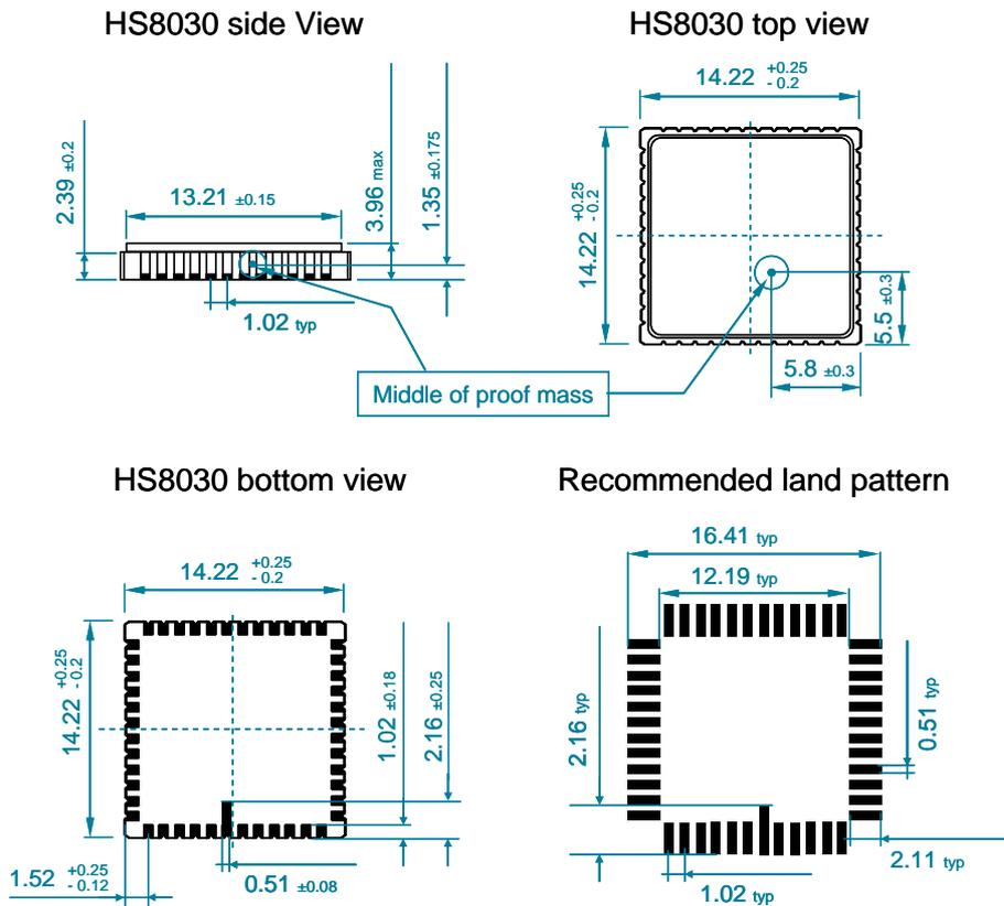
Figure 2: HS8030.D Packaging Size (all dimensions in mm)
