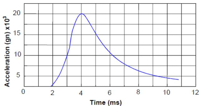
Figure 3: Typical gun hard shock profile
