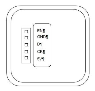
figure 2: Pinning of the ED-17-BB-512-S-P (bottom view)
