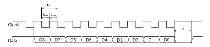
figure 3: SSI timing diagram
