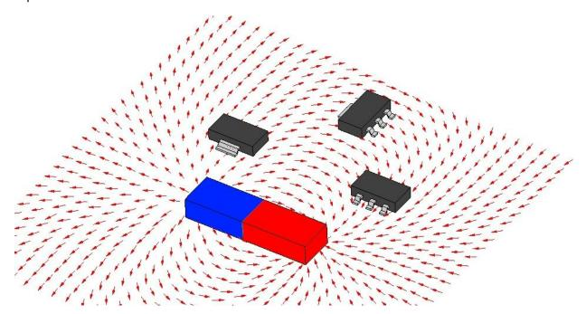
An uniaxial linear magnetic field will generate a linear output within the specified magnetic field range.
