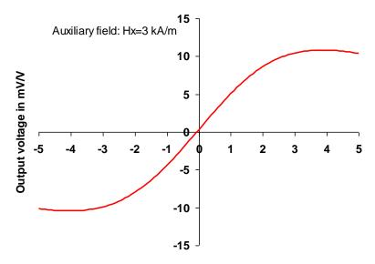
Figure 4: Characteristic output curve of KMY 20 S resp. KMZ 20 S for an auxiliary field strength of Hx=3 kA/m
