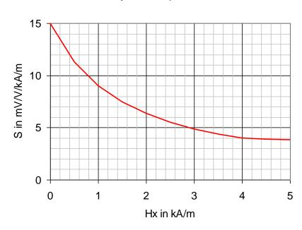
Figure 1: Sensitivity dependence on auxiliary field strength
