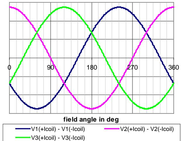
Figure 4: output voltage change due to coil influence
