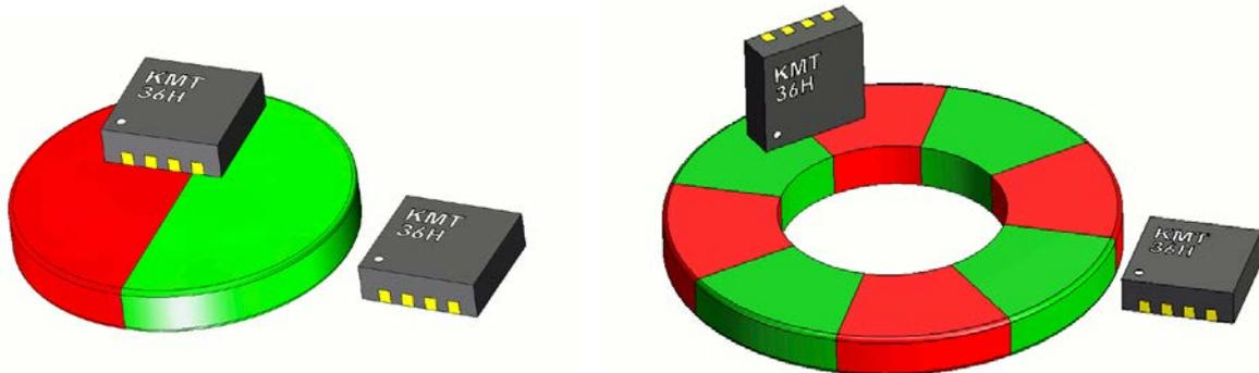
As an unique feature, the KMT36H is able to measure full 360° by utilizing an additional magnetic field which is generated by a planar coil that is integrated on the chip. The 180°/360° determination is done by a simple sign distinction and may be computed periodically or only once at power up.
