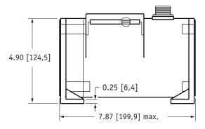
DIMENSIONS ARE IN INCHES [MM] tolerances are 0.03 IN. [0.5 MM] unless otherwise noted.
