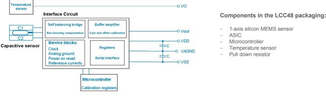
It is strongly recommended to use decoupling capacitors [C] of 1µF each between VDD and VAGND and between VAGND and VSS, placed as close as possible from the accelerometer. COG or X7R @ 5% capacitor types are recommended. On top, the VAGND track should be as short as possible. Any other setup will potentially affect the bias calibration and stability.
