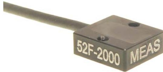
The **Model 52F** accelerometer has an advanced piezoresistive MEMS sensing element which offers excellent dynamic range and stability. This unit features a full bridge output with an operating temperature range from -40 to +90°C. A slight amount of gas damping provides outstanding shock survivability and a flat amplitude response to 7kHz.
