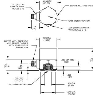
STANDARD TOLERANCE INCHES (MILLIMETERS) .XX = +/- .02 (.X = +/- .5) .XXX = +/- .010 (.XX = +/- .25)
