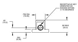
STANDARD TOLERANCE INCHES (MILLIMETERS) .XX = +/- .02 (.X = +/- .5) .XXX = +/- .010 (.XX = +/- .25)
